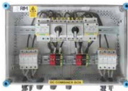
String Combiner box with Four inputs with String fuses and Two outputs with two isolators and two Surge protection devices
